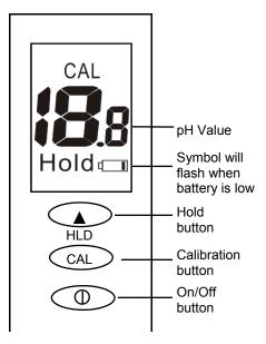
FIRST USE: If the unit fails to turn on, check that the batteries are working and properly installed.
